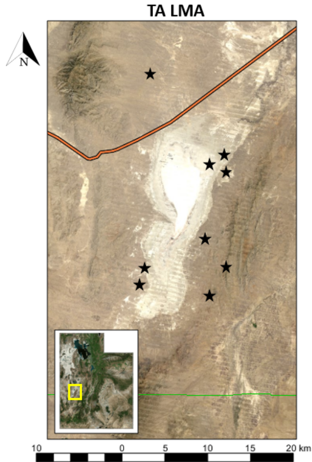
Figure 8. A map showing location of the TA LMA within the state of Utah. The black stars represent the individual LMA sensors. Graphic created using MATLAB.
